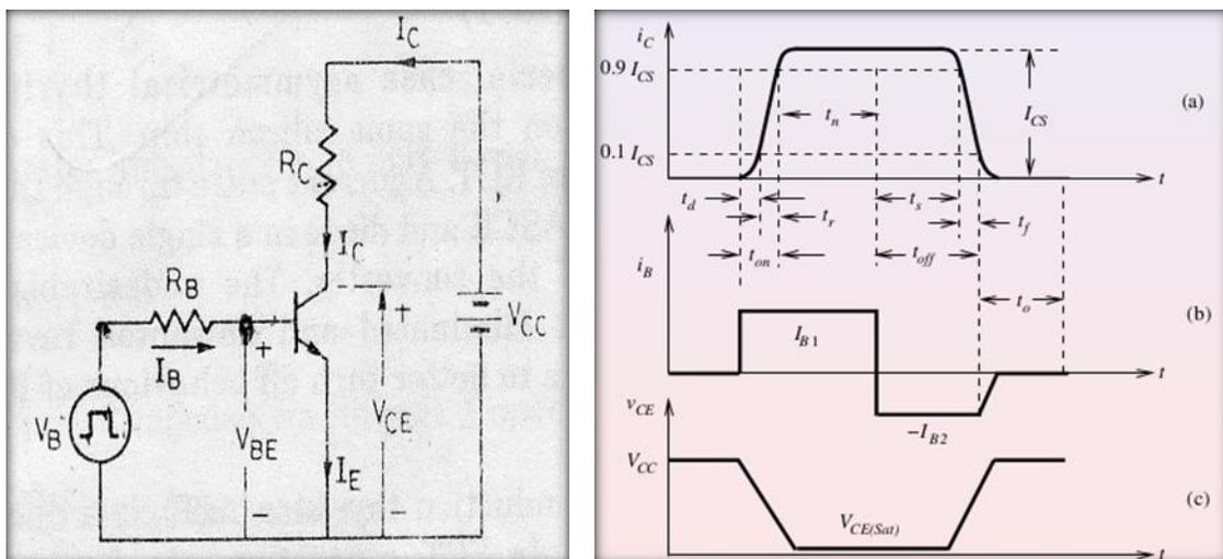
Fig.1 Switching Waveform of BJT
