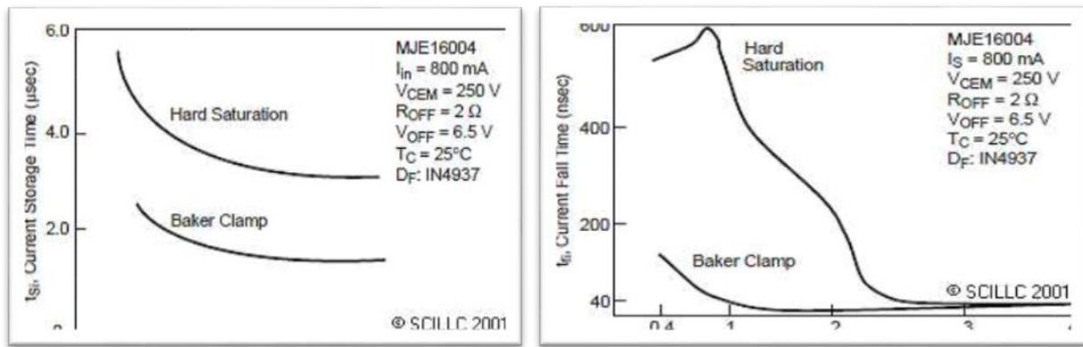
Fig. 3 Storage Time with Fixed Drive in a Baker Clamp Circuit & Fall Time with Fixed Drive in a Baker Clamp Circuit
