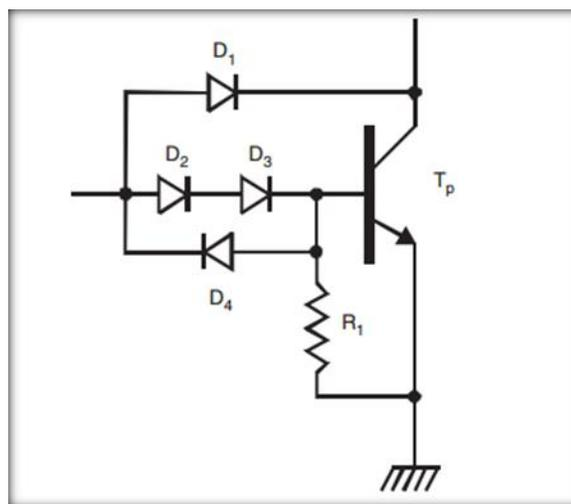
Fig. 2 Baker Clamp Circuit
