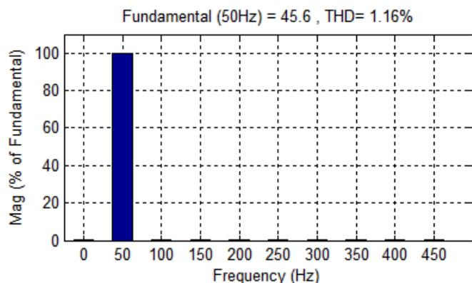
Fig. 8 FFT analysis of input current
