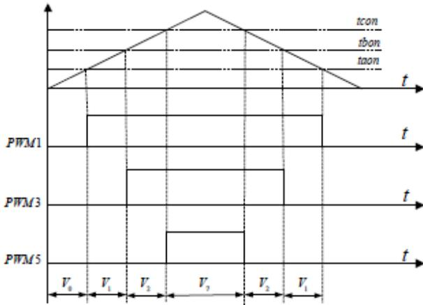
Figure 4 conventional and switching sequences in sector
