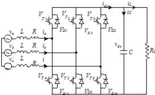
Figure 1. Circuit schematic of three-phase voltage source PWM rectifier.
