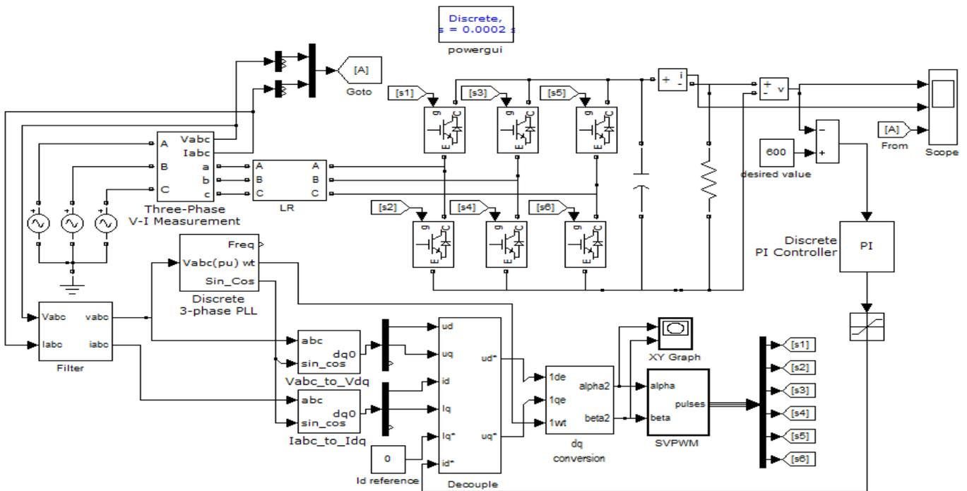
Figure 5 Three-phase Active Front End Rectifier simulation model
