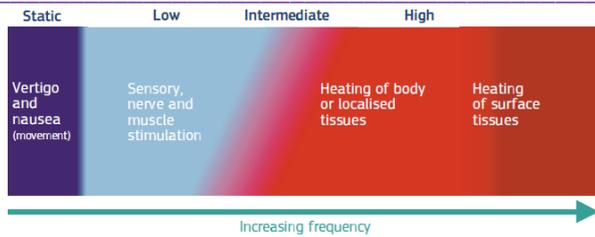
Fig. 4 Effect of EMI at Different Frequency Range
